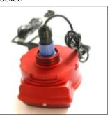
The battery begins charging as soon as it is connected to the charger.
