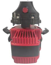
3. Push the hull cleaner electric brush down until it clicks into place, then close the clips on either side of the battery to lock it in place. The clips hold the battery pack in position and prevent it from detaching.
